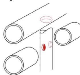
**2.** Holes for venting and draining should be diagonally opposite to one another at the high point and low point of the fabrication as it is suspended for galvanizing. Very long hollow sections may require additional vent holes to aid drainage and to help produce a better surface finish.
