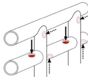
Sections can be interconnected using open mitred joints, or interconnecting holes can be drilled before fabrication. Pipe ends can be left open, or be plugged after galvanizing .
