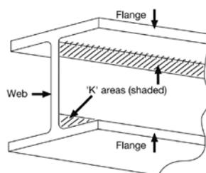
fabrication features into the 'K' areas of a section (where the web and flange meet) is unavoidable, please consult Galvanizers Association to discuss how best to finalise the design of the fabrication.
